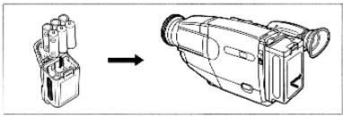
1. Insert six "AA" alkaline dry-cell batteries as shown, being sure not to confuse their polarity.
