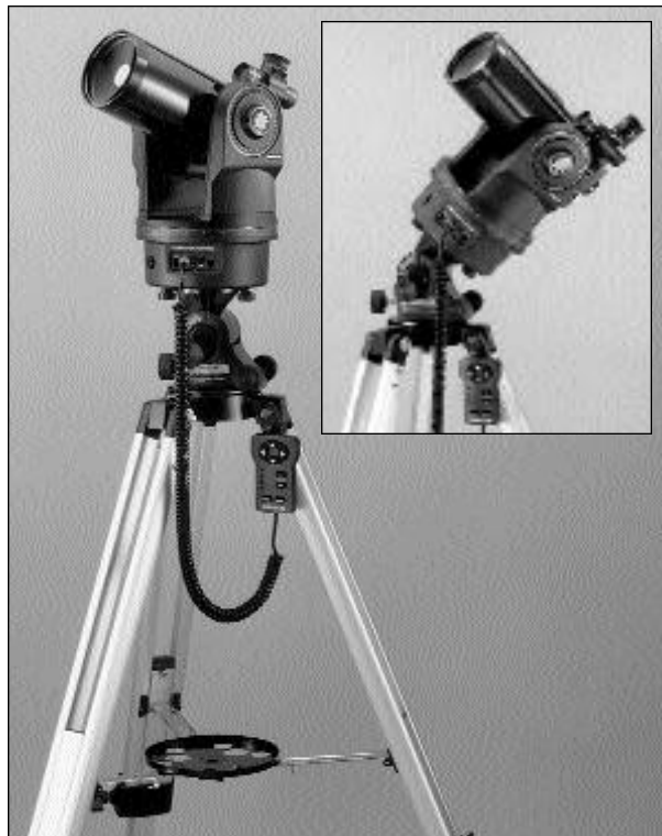
Fig. 29: The #883 Deluxe Field Tripod shown with an ETX-90EC Astro Telescope, set up in the Alt/Az configuration (tripod head locked at 90°), for terrestrial applications. (Inset) Tripod head tilted for polar alignment.
