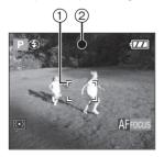
When you press the shutter button halfway, [AFFOCUS] indication disappears and then the aperture value and the shutter speed are displayed.
