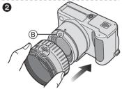
2 Rotate the ring © to the direction of the arrow until [LOCK] is adjusted to (A) on the adaptor.
