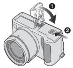
If the card/battery door cannot be completely closed, remove the card and insert it again.
