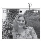
When the jitter alert appears, we recommend using a tripod. If you cannot use a tripod, be careful of how you hold the camera. (P33)
