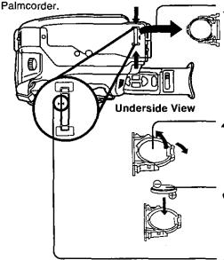
While pinching the stopper tabs, pull the tray out of the Battery Compartment.
