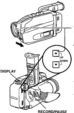
I While pressing the UP ▲ button, set the POWER swith to CAMERA.
