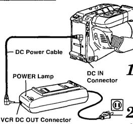
Connect the VCR DC OUT on the AC Adaptor to the DC IN on the Palmcorder with the DC Power Cable (supplied).
