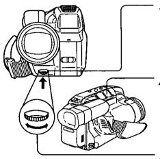
Press MANUAL FOCUS so that "MF" (Manual Focus) appears in the EVF. EVF Indication
