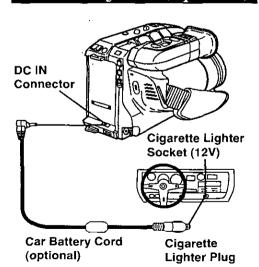
Connect a PV-C16 Car Battery Cord (optional) to the DC IN of the Palmcorder.
