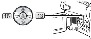
If the [ >>> ] Button [13] or [ <<< ] Button [16] is pressed during Playback, it turns to Cue Playback (A) or Review Playback (B).
