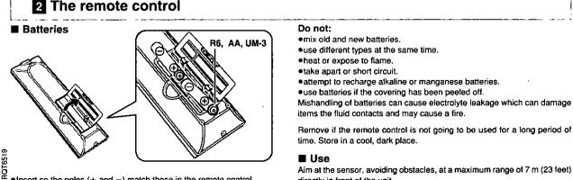
Insert so the poles (+ and -) match those in the remote control. Do not use rechargeable type batteries.
