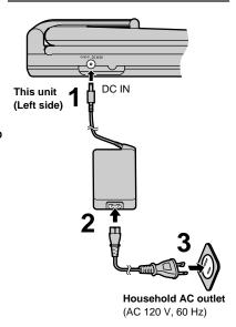
The unit is in the standby condition (the [6] indicator lights) when the AC power supply cord is connected. The primary circuit is always "live" as long as the AC adaptor is connected to an electrical outlet.
