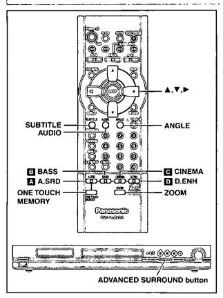
Use the ABCD buttons to control the following features, used to enhance your enjoyment of movies. ONE TOUCH CINEMA MEMORY then allows you to store the settings and recall them at a touch of a button. Turn ADVANCED SURROUND and BASS PLUS off when using Dolby Pro Logic. Dolby Pro Logic will not work correctly if they are on.
