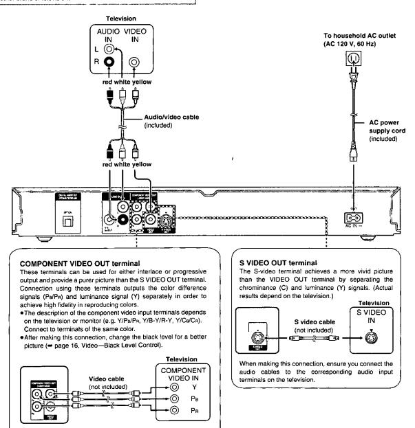
When making this connection, ensure you connect the audio cables to the corresponding audio input terminals on the television.
