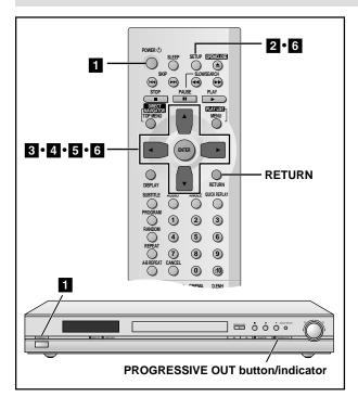
The **QUICK SETUP** screen appears when you press [SETUP] the first time after purchase and assists you to make necessary settings. You can access this screen again later if you need to ( → page 21, Others—QUICK SETUP).
