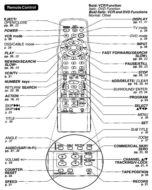
**EJECT button:** When this button is pressed in VCR mode, the tape is ejected. This button is inoperative if pressed during recording. If pressed in DVD mode, the disc tray opens or closes.
