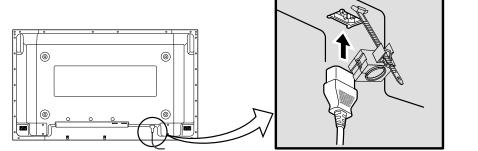
Fix the AC cord plug securely to the Plasma Display with the clamper. (See page 9)
