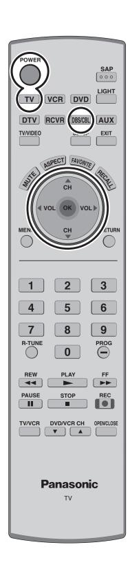
1 TV Press to operate the TV set with the remote control.
