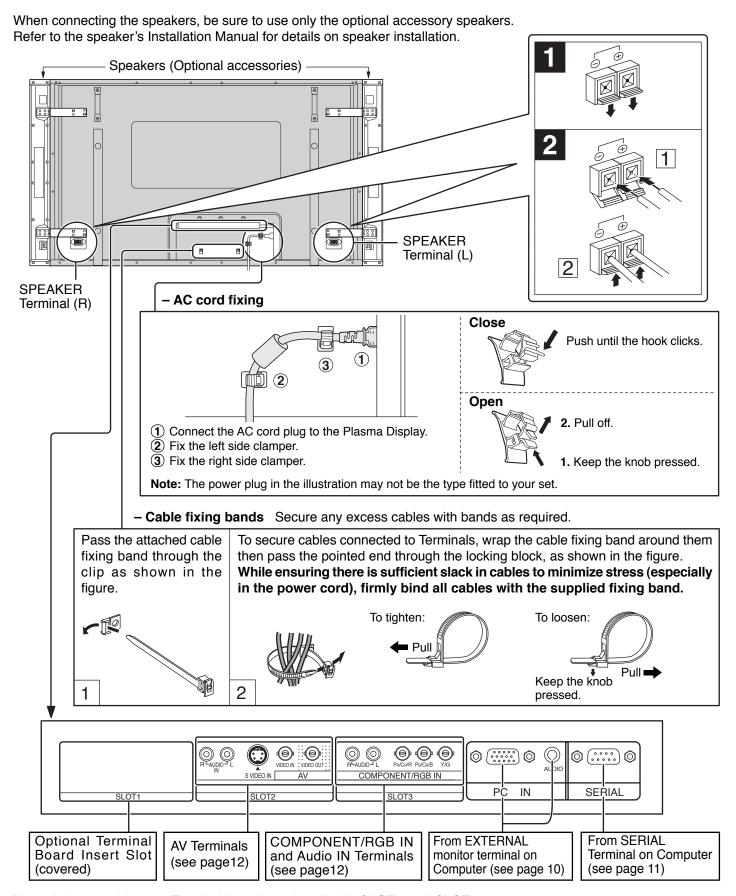
**Note:** At factory shipment, Terminal boards are installed in SLOT 2 and SLOT 3.
