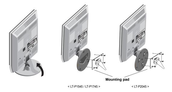
Align the mounting interface pad with the holes in the rear cover mounting pad and secure it with the four screws that come with the arm-type base, wall mount hanger or other bases.
