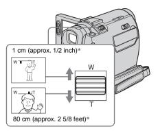
\* The minimum distance required between your camcorder and the subject to get a sharp focus in that position of the lever.
