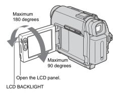
Open the LCD panel 90 degrees to the camcorder, then rotate it to the desired position.
