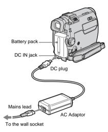
**1** Attach the battery pack by sliding it in the direction of the arrow until it clicks.
