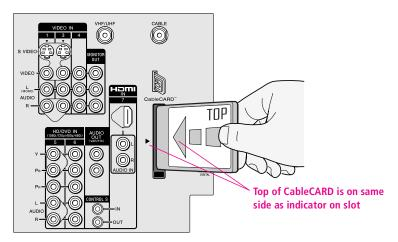
CAUTION: Inserting the CableCARD incorrectly may result in permanent damage to the card and the TV.
