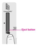
**2** Pull the CableCARD straight out of the slot to remove it. To install a different CableCARD, follow the instructions in "Activating CableCARD Service" on page 41.
