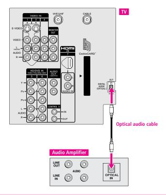
Because all equipment does not output digital audio, you should also connect the TV's analog audio output jacks to the amplifier's analog audio input jacks, as described on page 36.
