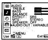
**VARIABLE:** Sound output varied according to the projection TV settings. You can adjust the volume, bass, treble, and balance.
