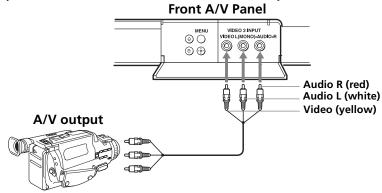
If you have an S VIDEO equipped camcorder, you can use an S VIDEO cable for optimum picture quality (KV-27FV17 only).
