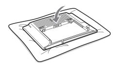
2 Slide the LOCK/UNLOCK latch on the back of the monitor to the UNLOCK position. From the bottom of the compartment, slide the battery into the monitor until it clicks into place.
