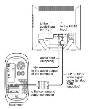
When connecting a Macintosh computer, use an adapter (not supplied), if necessary. Connect the adapter to the computer before connecting the video signal cable.
