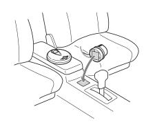
1 Attach the supplied Velcro tapes to the bottom of the rotary commander and to a flat place.
