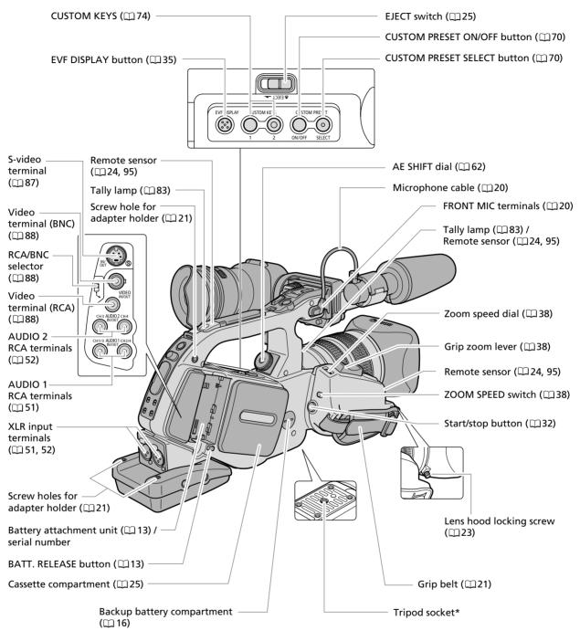
\* Do not use tripods with fastening screws longer than 0.2 inch (5.5 mm) as it may damage the camcorder.
