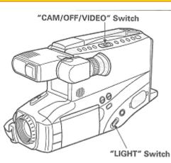
3. After use, set "LIGHT" to "OFF' or set "CAM/ OFF/VIDEO" of the camcorder to "OFF" position.
