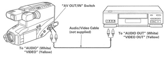
**NOTE:** When dubbing the sound and picture from a video source, set "**AV OUT/IN**" to the "**IN**" position. When dubbing the sound and picture from the camera, set "**AV OUT/IN**" to "**OUT**" and do not connect "**AUDIO**" and "**VIDEO**" jacks.
