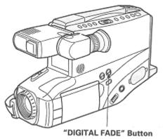
**NOTE:** When fading out be sure to wait until the PAUSE indicator ( $\square$ ) is visible in the viewfinder before attempting to put the camcorder into the record mode again.
