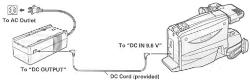
1. Plug the AC adaptor/charger power cord into AC electrical outlet.
