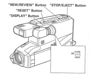
NOTE: The tape will also stop approximately at "0000M" during fast forward mode.
