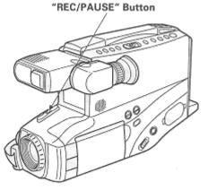
7. Press **"REC/PAUSE"** to stop recording. Press the button again to resume recording. The "—" indication will appear in the viewfinder or on the LCD monitor instead of **"REC"** while the camcorder is in the record/pause (stand-by) mode.
