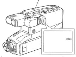
**NOTE:** When **"DISPLAY"** is pressed and **"INDEX"** is displayed in the viewfinder or on the LCD monitor, an **"INDEX"** signal is recorded when recording is started, and when the **"INDEX"** signal has been recorded, **"INDEX"** disappears.
