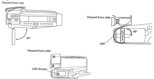
• If the LCD monitor is turned 90° so that it faces the same direction as the lens when the camera signal is being recorded during recording, recording pause, instant review, editing, A/V dubbing or A/V dubbing pause, the image on the monitor screen will become a mirror image, and the viewfinder will turn on. The on-screen display on the LCD monitor will also be as if reflected on a mirror.
