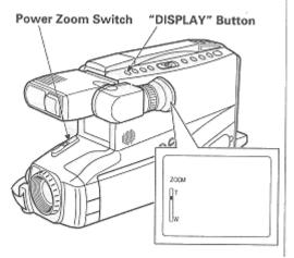
**NOTE:** When the digital zoom is used, the more the image is magnified, the rougher the picture becomes. Also even a slight shaking of the camcorder is conspicuous.
