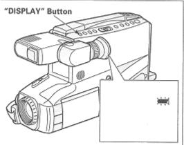
Press the "DISPLAY" button. The remaining battery power level will appear in the viewfinder.
