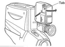
To replace the front case, pass the lamp through the hole of the reflection plate then attach the upper hooks to the camera light, and then attach the lower hook to the camera light.
