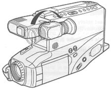
. You can adjust the position and angle of the viewfinder so you can see through it easily.
