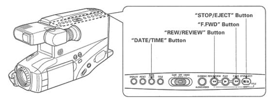
1. Press and hold the small button on "CAM/OFF/ VIDEO", and then slide it to "CAM" position.
