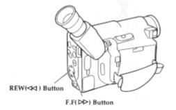
**Note:** When you engage F.F button or REW button the picture will have some interference or noise. This is normal during search mode.
