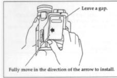
3. Once the arrows are aligned, push down on the battery.
