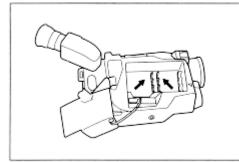
3. Insert six alkaline batteries with the correct polarities.
