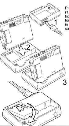
Plug the power cord into the back of the charger unit (1). Plug the other end of the cord into a live household outlet. The included AC cord is designed for the current of the sales region. Only use the cord in the region it was purchased. For more on the AC cable, see page 104.
