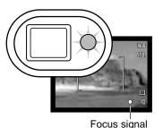
**Focus confirmed** - the LCD monitor focus signal is white, the viewfinder indicator lamp is green and steady. Focus is locked.
