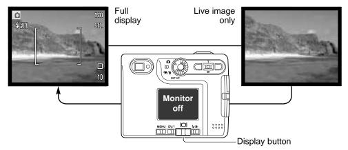
Battery power can be conserved by turning the monitor off and using the viewfinder to take pictures. However, because of parallax, the monitor should be used for subjects closer than 1m (3ft.) at the zoom lens' wide-angle position or 3m (10ft) at the telephoto position.
