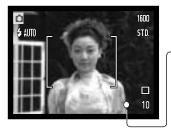
Place the subject within the monitor focus frame or center the subject in the viewfinder. Press and hold the shutterrelease button partway down to lock the focus.
