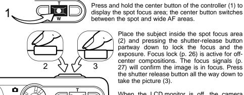
display the spot focus area; the center button switches between the spot and wide AF areas. Place the subject inside the spot focus area
