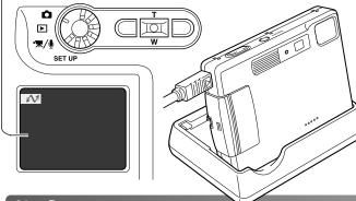
The charger can be used as a camera stand. When the camera is on, the charger does not charge or supply power to the camera.
