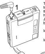
The AC adapter AC-4 or AC-5 allows the camera to be powered from a household outlet. The AC adapter is recommended when the camera is interfaced with a computer or during periods of heavy use. AC adapter model AC-4 is for use in North America. Japan, and Taiwan, and AC-5 is for use in all other areas. The battery cannot be charged using the AC adapter.
