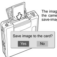
The image in the buffer memory can be saved. Without turning the camera off, insert a new memory card into the camera; a save-image message will be displayed.
