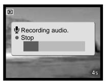
A status bar and the frame counter displays the remaining recording time. The audio caption can be stopped during the fifteen-second recording period by pressing the central button of the controller (1).
