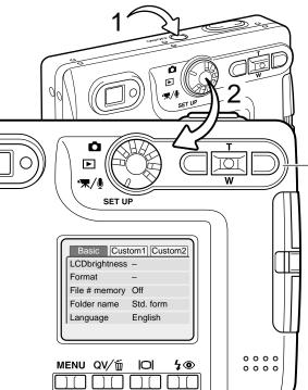
Turn the camera on by pressing the main switch near the shutter-release button (1).
