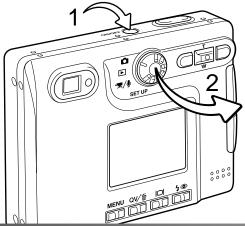
Turn the camera on by pressing the main switch near the shutter-release button (1).
