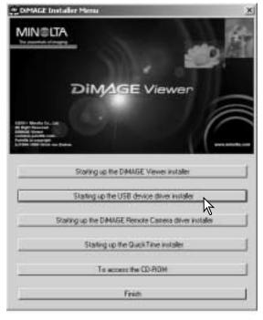
Before connecting the camera to the computer, place the DiMAGE Viewer CD-ROM in the CD-ROM drive. The DiMAGE installer menu should automatically activate. To automatically install the Windows 98 USB driver, click on the starting-up-the-USB-device-driver-installer button. A window will appear to confirm that the driver should be installed; click "Yes" to continue.
