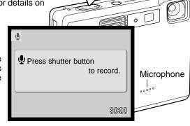
To begin recording, press and release the shutter button (1). The frame counter will display the elapsed time; during the last ten seconds, the counter will turn red and count down the time. The recording will stop when the shutter-release button is pressed again or the remaining time has elapsed.
