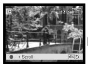
Pressing the up key increases the image magnification. Pressing the down key decreases the image magnification.
