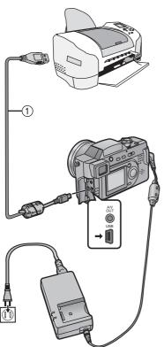
By connecting the camera to a printer corresponding to USB DIRECT-PRINT via the supplied USB connection cable, it is possible to print directly.
