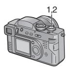
If the subject is out of the AF area and you press the shutter button, the subject's focus is not adjusted. After locking focus and exposure (AF/AE lock), you can take a clear picture with adjusted focus. AF: Auto focus
