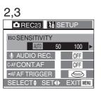
The ISO setting adjusts the camera's sensitivity to light. Generally, the lower the ISO setting, the better the picture quality will be. Increasing the ISO value will make the camera more sensitive in low light.
