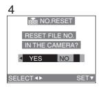
As the file numbers are recorded sequentially by the camera, when you use two or more cards, it may happen that the file numbers on your cards do not start from 0001. Use this function when you insert a new card or perform a new recording on the recorded card and you want to start recording from the file number 0001.
