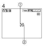
When this mode is selected, both the focus and the exposure will be adjusted to spot on a limited area. This is suitable when you take pictures in delicate light conditions and intend to take a picture in a limited area.
