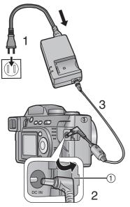
If you use an AC adaptor as indicated in 3, you can use the camera without worrying about battery discharge.
