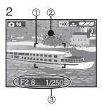
By only pressing the shutter button, the exposure (shutter speed and aperture value) will be automatically adjusted and the picture will be taken.
