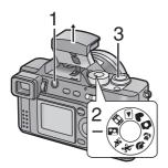
The Night Portrait mode combines the electronic flash with a "slow shutter" mode. This unique feature allows you to photograph close subjects against the natural night background. Since the shutter speed is slow, we highly recommend using a tripod to steady the camera.
