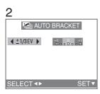
Pressing the shutter button once, the camera will automatically take 3 pictures changing exposure according to the set exposure compensation value.
