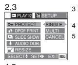
4,5 (1) © ¬PROTECT THIS [722] 100-0001 1/10 SELECT <► SET▼ EXITER Using this feature, important photos can be protected from accidentally being deleted. This feature cannot protect photos or any data on the Card if the entire card is formatted.
