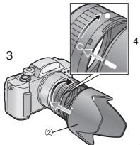
When using the camera in bright sunlight, the lens hood should be installed. This will minimize lens flare and ghosting, thus improving the overall quality of the photo.
