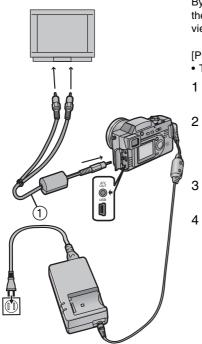
By connecting the camera to a television via the supplied A/V cable ①, it is possible to view and play back the recorded images.
