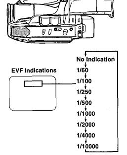
**1** Press HIGH SPEED SHUTTER while recording.
