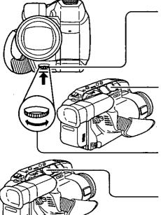
Press MANUAL FOCUS so that "MF" (Manual Focus) appears in the EVF. EVF Indication
