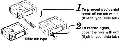
To prevent accidental erasure, break off the tab with a screwdriver. (If slide type, slide tab open.)
