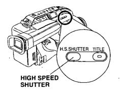
Press HIGH SPEED SHUTTER while recording.
