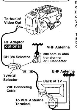
If TV has no VIDEO/AUDIO IN jacks, connect PV-RF16 RF Adaptor (optional, page 80). Tune TV to CH 3 or 4 to match RF Adaptor CH 3/4 Selector. Set Adaptor's TV/VCR Selector to VCR for playback.
