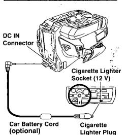
Connect PV-C16 <u>Car Battery Cord</u> (optional, page 80) to <u>Camcorder</u> DC IN.
