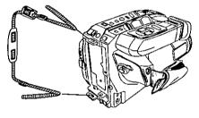
Thread strap ends through Strap Rings on Camcorder.
