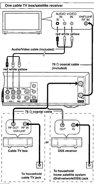
When a home satellite system (Dishnetwork/DSS) is connected, auto tuning and auto clock setting may not operate properly. Set the clock manually (→page 13).
