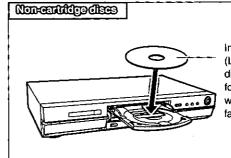
Insert label-up. (Load double-sided discs so the label for the side you want to record is facing up.)
