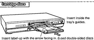
so the label for the side you want to record is facing up.) • When using 8 cm (3") DVD-RAM, remove the disc from the
