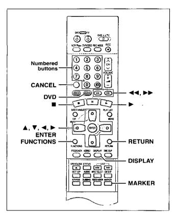
You can mark positions by pressing [MARKER]. Also use on-screen menus to mark, recall, and clear positions.
