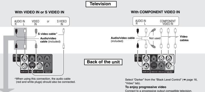
You can connect the audio cable to the 2channel audio input terminals of an analog amplifier or system component to enjoy stereo sound. Connect to a progressive output compatible television.
