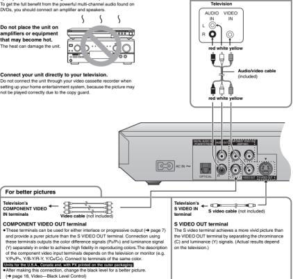
When making this connection, ensure you connect the audio cables to the corresponding audio input terminals on the television.
