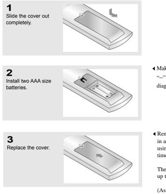
Make sure to match the "+" and "-" ends of the batteries with the diagram inside the compartment.
