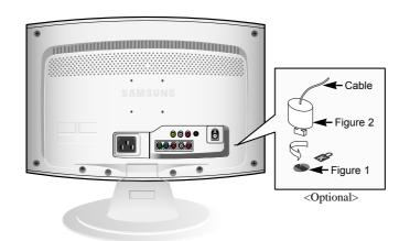
The Kensington lock is a device used to physically fix the system when using it in a public place. The locking device has to be purchased separately. The appearance and locking method may differ from the illustration depending on the manufacturer. Please refer to the manual provided with the Kensington lock for proper use.
