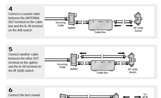
cable between the OUT terminal on the RF (A/B) switch and the VHF/UHF terminal on the rear of the TV. After you've made this connection, set the A/B switch to the "A" position for normal view
