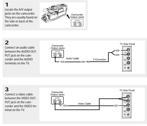
The audio-video cables shown here are usually included with a Camcorder. (If not, check your local electronics store.) If your camcorder is stereo, you need to connect a set of two cables.
