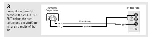
The audio-video cables shown here are usually included with a Camcorder. (If not, check your local electronics store.) If your camcorder is stereo, you need to connect a set of two cables.
