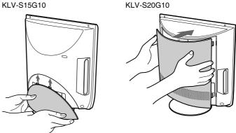
**2** Push the two tabs of the lower side of the rear cover into the square holes of the TV.
