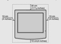
When installing the unit using a stand, allow this much space.
