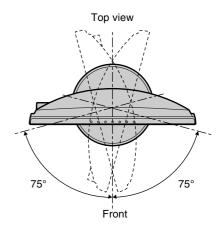
Mhen adjusting the angle, hold the stand with one hand to avoid slipping or tipping the stand.
