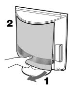
Do not carry the TV holding the rear cover only as the rear cover is easily removed.
