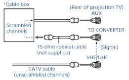
For this set up, you can switch between scrambled channels (through your cable box), and normal (CATV) channels by pressing ANT on your remote control.
