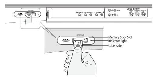
Be sure to insert the Memory Stick in the correct direction. If the Memory Stick is forced in the wrong way, it may become damaged.
