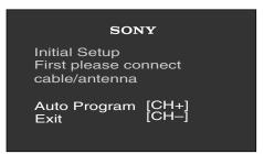
Press  $\stackrel{\text{CH}}{\div}$  on the remote control or on the TV front panel to start Auto Program, or press  $\stackrel{\text{CH}}{\hookrightarrow}$  to exit.
