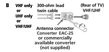
Converter EAC-25 is commercially known as a 300-to-75 ohm antenna adapter.
