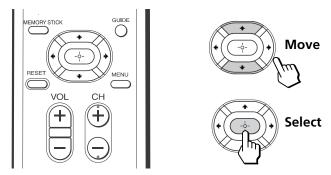
To navigate on the on-screen menus, use the arrow buttons  $(\diamondsuit, \heartsuit, \diamondsuit, \diamondsuit)$  to move the cursor. Pressing these arrows will cause the cursor to move in the corresponding direction. Press the center button  $(\textcircled{\Rightarrow})$  to select an option.
