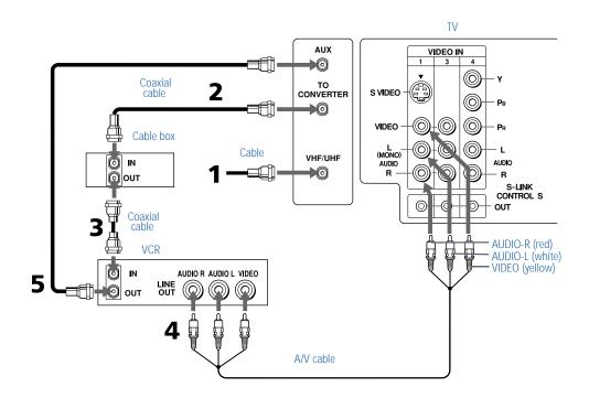
Pressing the ANT button on the remote control switches between the channels coming in through the cable box (scrambled) and those coming directly to the TV (unscrambled).
