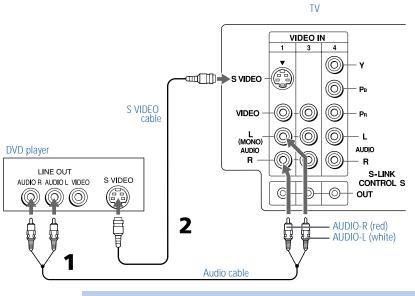
Use the TV/VIDEO button on the remote control to switch between the VCR, DVD player and cable TV inputs.
