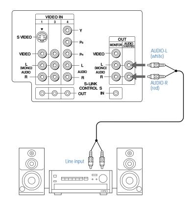
1 Using audio cables, connect the TV's Audio OUT jacks to the audio receiver's Audio LINE IN jacks.
