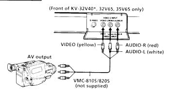
\* KV-32V40 does not have S VIDEO on the front panel.
