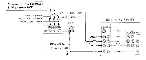
The S-Link connector must be in the same VIDEO-IN jacks as the A/V cables on your TV.
